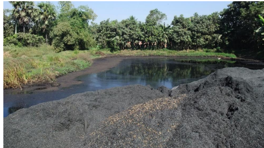
Solid and liquid wastes from gasification system at Yam Chan rice mill, Battambang province, Cambodia, 2014 - 12 - 20
