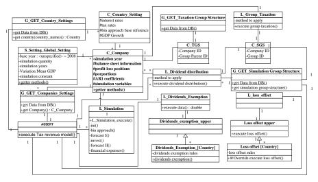
Fig. 4. Illustration of the ASSERT model in UML
