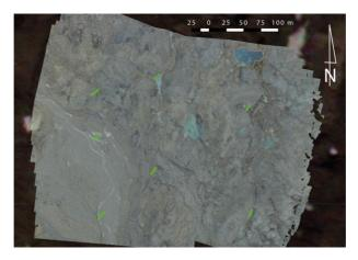
FIG. 5. Assessment of the discrepancies using two different software programs on the same dataset. The orthophotograph of the area under consideration has green lines indicating the shift between features found on the two orthophotographs generated using IGN MicMac and Agisoft PhotoScan. This is generated from the same dataset of photographs annotated with the same GNSS positions found in the Exif header. The typical shift (green lines) is 10 m.
