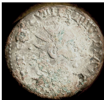
Fig. 16. Silver coin 34015_C01 under treatment. Most of the corrosion has been removed with acid citric bath and the rest is treated mechanically. Part of the red and green corrosion layers are still visible.
