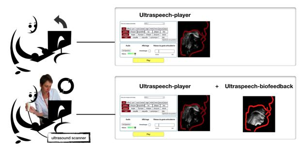
**Figure 1**. Top: illustration of the control interface and midsagittal ultrasound image display with sketchy vocal tract outline provided by *Ultraspeech-player* and used in the *IL* protocol. Bottom: illustration of the double interface, including the real time display of the speaker's tongue by *Ultraspeech-biofeedback*, used in the *FB+I* protocol.
