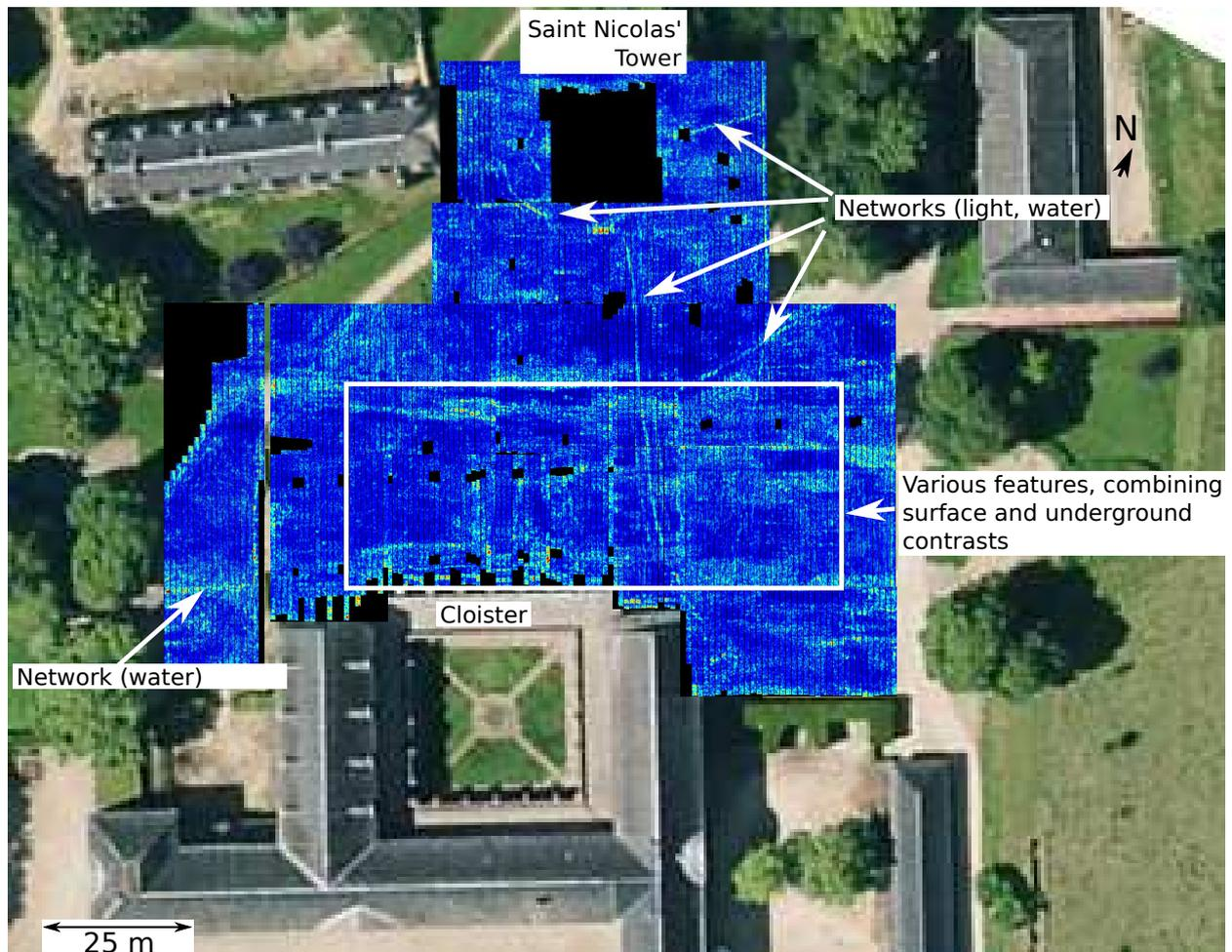
Figure 5: GPR slice at 0.3 m depth.
