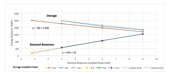
Figure 7: Energy displaced by Storage and Demand Response as a function of installed power of Storage and DR
