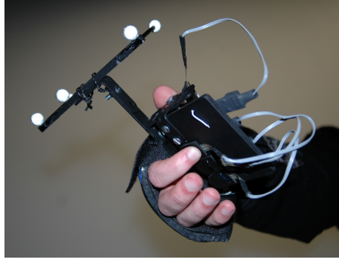
Figure 7. The Piivert device feature pressure sensors for each finger, which enable percussion gestures and expressive excitation gestures to be performed in combination with graphical 3D interaction techniques.
