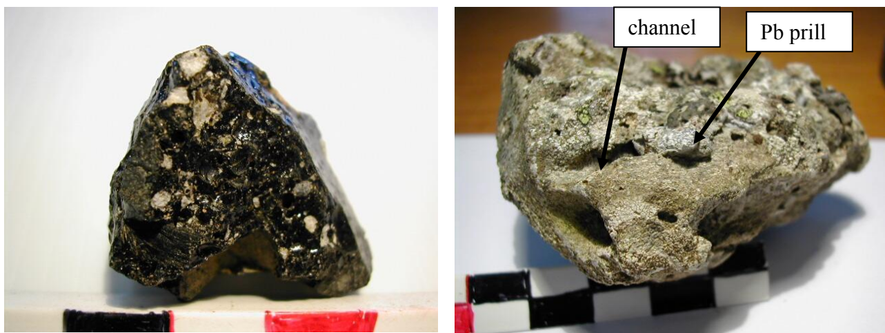
Fig. 5 (left) : black glassy slag, with quartz and feldspar inclusions.
