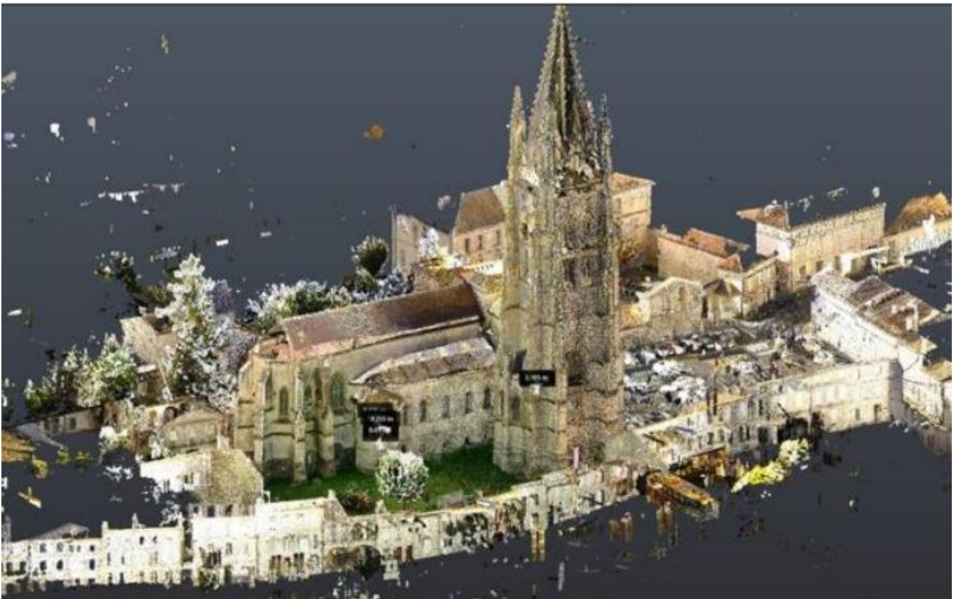
Figure 4: Perspective view of the Basilica Sainte Eutrope – Points cloud from a photogrammetric survey – Saintes (France) – Archeovision
