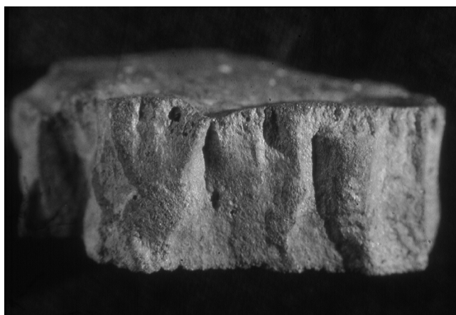
Figure 7: Side view of a slag fragment as found, showing the typical prismatic layer of 1-2mm below the upper surface (total thickness ~10mm)
