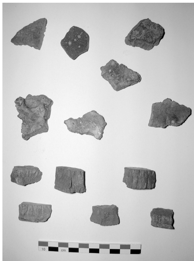
Figure 6: Slag fragments from Early Bronze Age sites in the Saint-Véran mining district, exhibiting the typical Plattenschlacke morphology.
