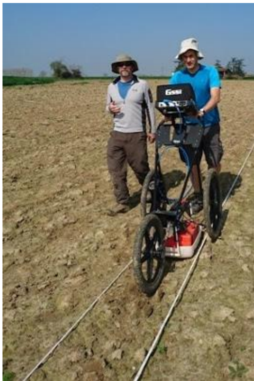
Figure 31 - GPR SRI 4000 (GNSSI) – (Photo. N. Poirier)
