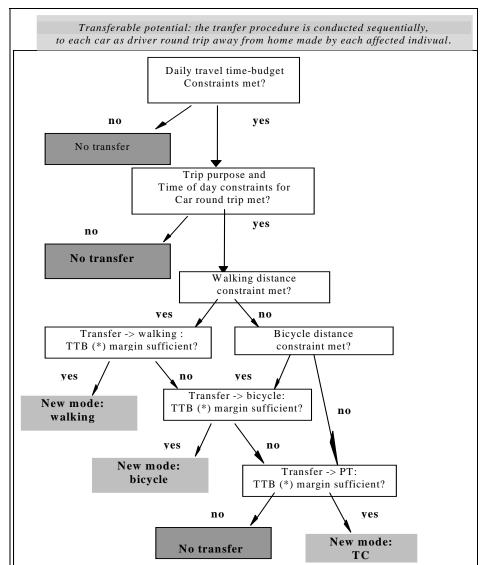
Figure 1: Simplified modal transfer procedure of individual car tour or round trip
