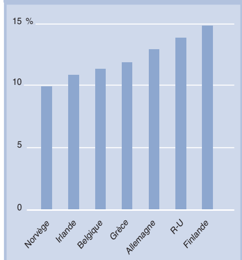
Figure 25 : Contribution des gains solaires passifs Source : NTNU, Norwegian University of Science and Technology
