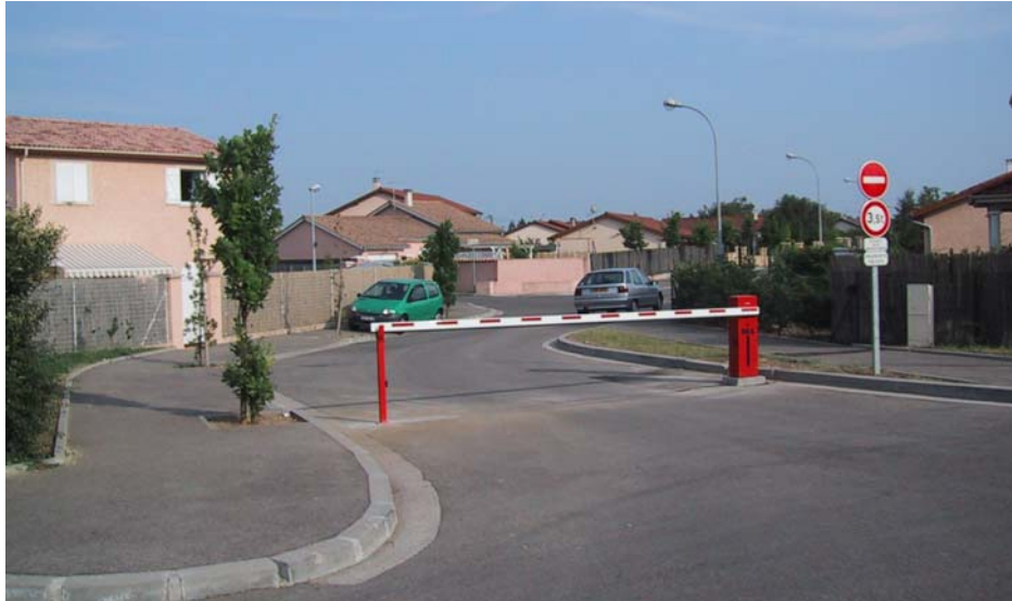
Figure 2. A gate in front of a French outer suburban estate designed to prevent drivers to use the street as a shortcut. The design of the barrier shows that security is not a major concern.
