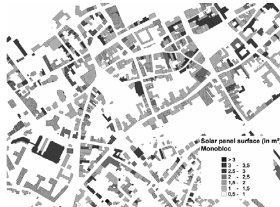
Figure 3: Solar panel surface (m 2 ) necessary to meet 50% of individual needs for domestic hot water (applied to the town of Compiègne)
