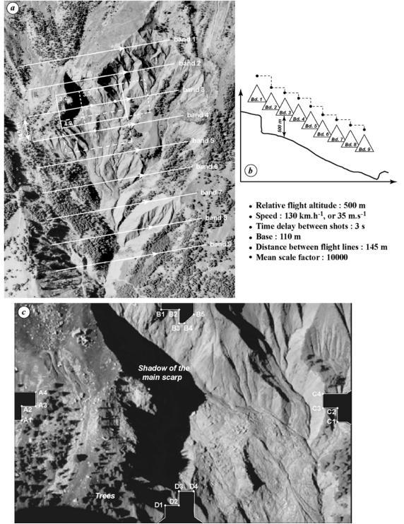
Fig. 4 – Flight paths (a) and decreasing altitudes (b). Example of a photography (c) with four fiducial marks (noted A1-A4, B1-B5; C1-C4; D1-D4)
