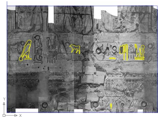
Figure 9. Epigraphic survey on the developed surface of a column of the Karnak Hypostyle Hall
