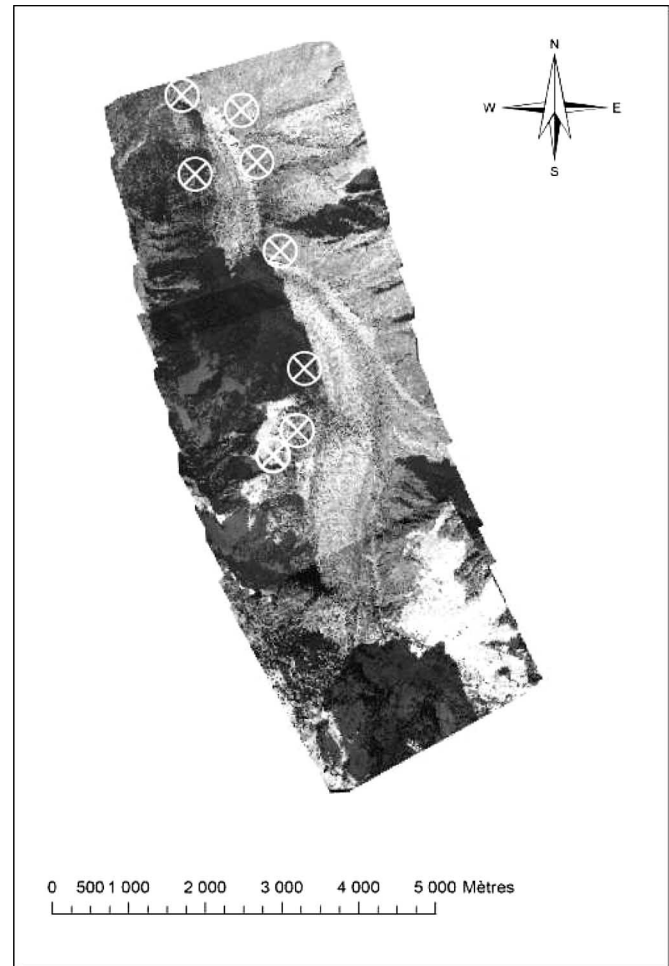
Fig. 3. Layout of the set of 13 photos that were taken over the Mer de Glace in 1995 and are entering in the AT processing. Circles represent the points measured by GPS.
