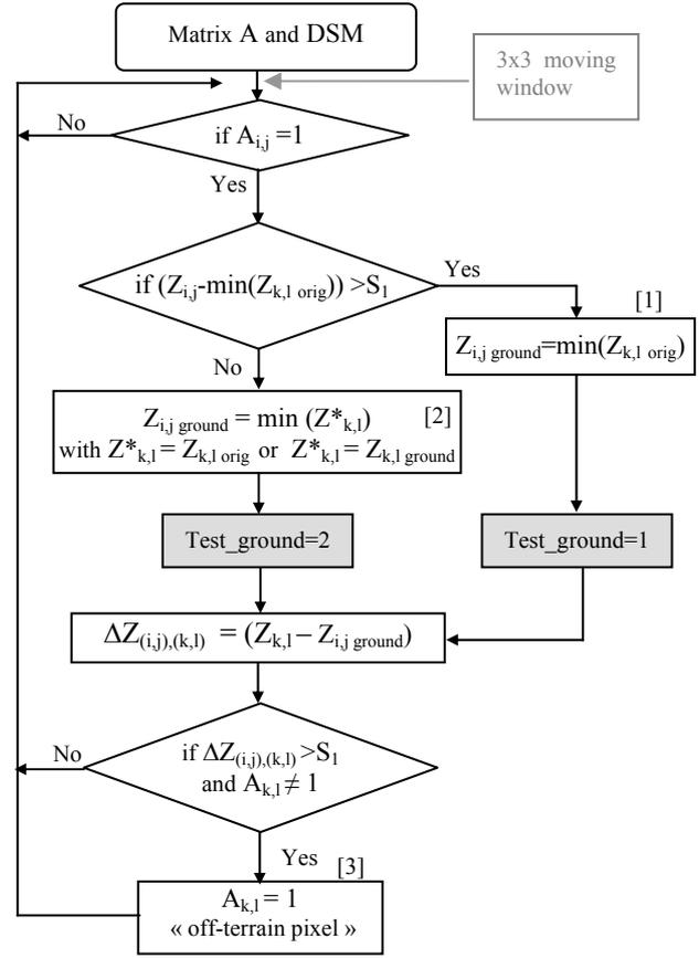
Figure 3. Workflow for the detection of off-terrain pixels
