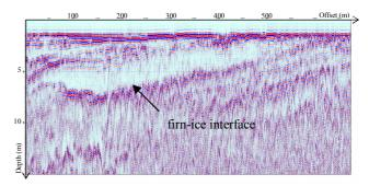
Figure 3. Longitudinal profile observed by GPR in 250 MHz frequency
