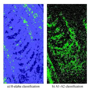
Figure 2. Early classification performed on PolSAR H-alpha and PolInSAR A1–A2 features resulting from coherence optimisation. Use of conventional feature space partitioning and color tables after PolSARpro software.
