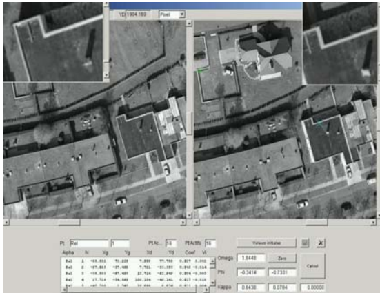
Figure 2. Optional additional views (zoom) for each image, as an example in the window of relative orientation.
