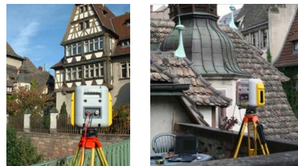
Fig. 10. Trimble GX scanner during the survey
