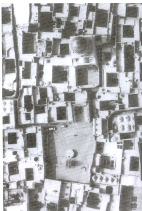
F.2: The concentrate urban form reduces penetration the dusty wind as far as influence of hot radiation on the surface. (Source of photo: Urban construction in arid and hot zones, 2002)
