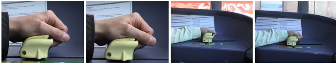
Figs. 1–4 Standard throttle with dead-man device: two operator positions, for activating the dead-man device and traction
