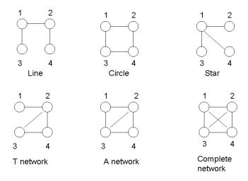
Figure 1: The six 4-player connected architectures
