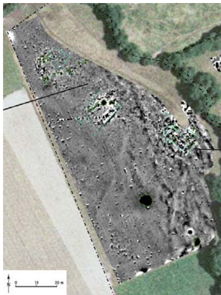
Magnetic prospection on the site of Roull (scale -9 to 9 nT/m) : orthophotography ( administrative limits and anomalies.
