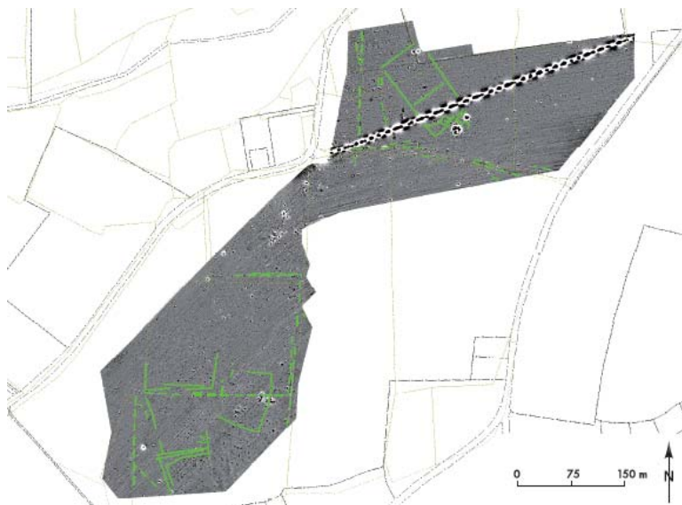
Magnetic prospections over 17 ha in the South of the city and land registers (scale = \pm 4 nT/m) : the administrative layouts are perfectly visible. One observes a division of the central piece former to the Napoleon's register and a small shift between the administrative layout and the corresponding magnetic anomaly.
