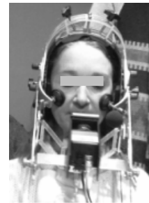
Figure 1: Helmet fixed on the head with camera mounted in front of the mouth, head-mounted microphone and US fixed under the chin.
