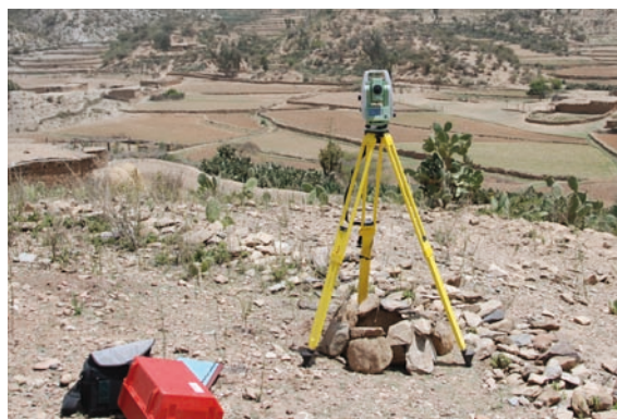
Figure 3: Total station Leica Flexline TSo6 (IG 2011).
