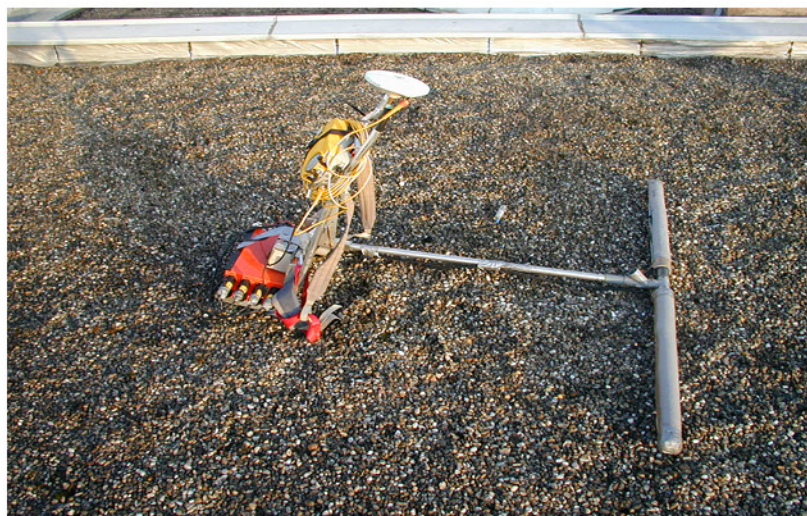
Antenna and GPS receiver
