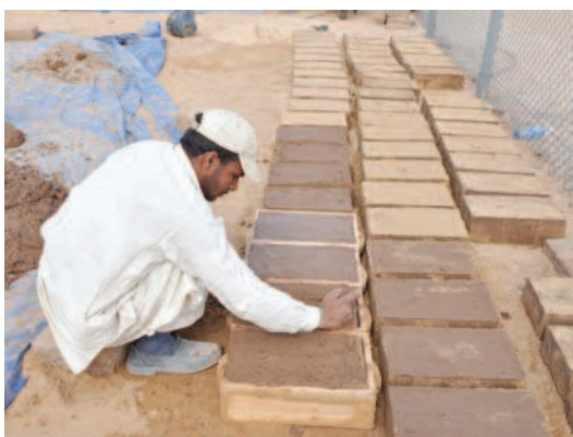
Fig. 13.15 Smoothing the surface of the earth in the mould
