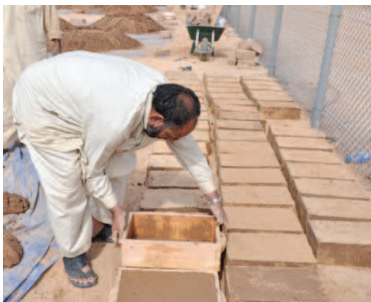
Fig. 13.16 Removal from the mould
