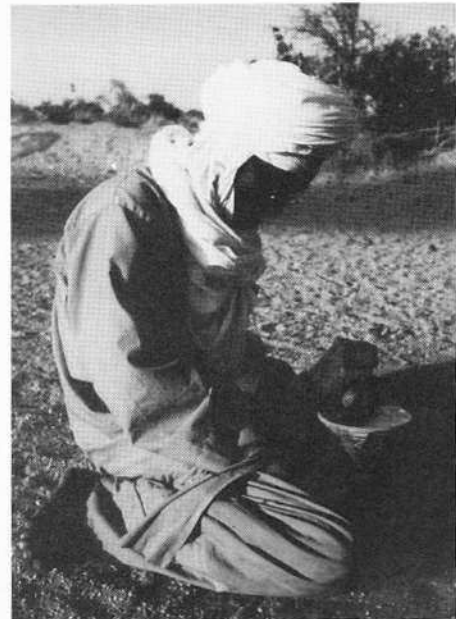
Fig. 7 Tuareg blacksmith grinding charcoal on a wooden mortar turned upside-down.
