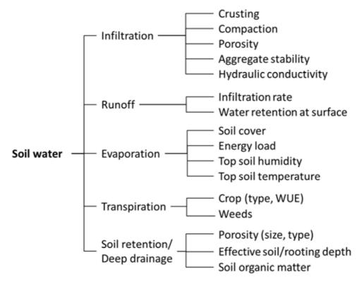
Figure 6.1 Processes and parameters affecting soil water
