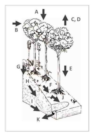
**Fig. 2.2.** Hydrological pathways are shown within a forested hillslope schematic, but present at scales from 0.1 km<sup>2</sup> experimental basins to international basins covering millions of square kilometres. Adapted by NA Chappell from the original diagram by Nick Scarle (with permission) published in Douglas (1977) Humid Landforms. MIT Press.
