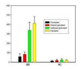
Fig. 2.13 Example of differences in slope erosion (ER) between undisturbed forest and cropland (labelled as 'farmland') by Liu *et al.* (2005 J. Mt. Sci-Engl: 2: 68-75). The runoff coefficient (RC) is also shown.
