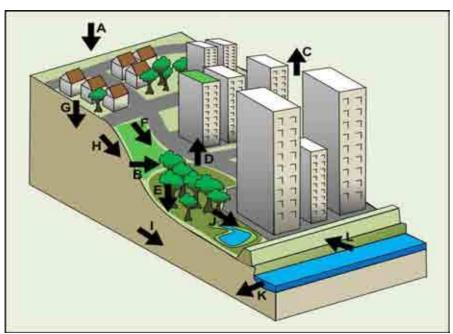
**Figure 5.2. Flow paths in urban areas.** (A=rainfall/snowfall; B=cloud-water interception; C=evaporation; D=transpiration; E=throughfall/stemflow; F=infiltration-excess overland flow; G=infiltration; H=lateral subsurface flow in soil strata; I=lateral subsurface flow in regoilith/rock; J=saturation overland flow; K=river/channel flow; L=overbank inundation).
