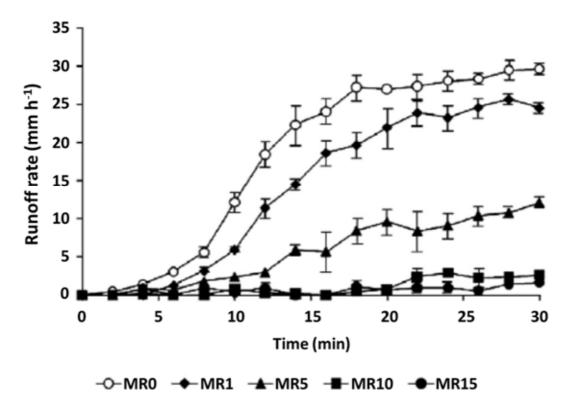
**Figure 632** Variation of mean run-off rates under different mulching rates. MR0=control; MR1=1 Mg ha<sup>-1</sup> year<sup>-1</sup>, MR5=5 Mg ha<sup>-1</sup> year<sup>-1</sup>; MR10=10 Mg ha<sup>-1</sup> year<sup>-1</sup>; MR15=15 Mg ha<sup>-1</sup> year<sup>-1</sup>. N=5 for each mulching rate treatment. Vertical bars indicate ± standard deviation (Jordan et al. 2010)
