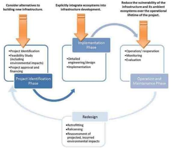
Figure 8.1. Proposed actions for how natural infrastructure can be mainstreamed into engineering water infrastructure (source: Mathews *et al* 2011).
