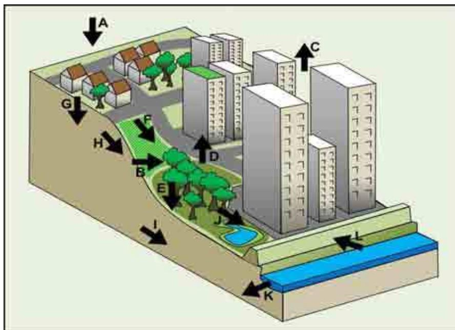
**Figure 5.2. Flow paths in urban areas.** (A=rainfall/snowfall; B=cloud-water interception; C=evaporation; D=transpiration; E=throughfall/stemflow; F=infiltration-excess overland flow; G=infiltration; H=lateral subsurface flow in soil strata; I=lateral subsurface flow in regolith/rock; J=saturation overland flow; K=river/channel flow; L=overbank inundation).
