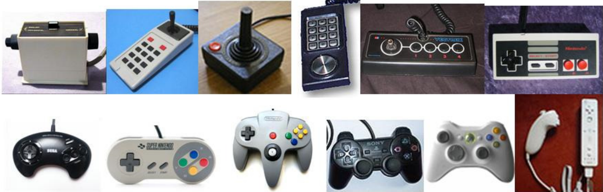
Figure 1. From left to right, top to bottom illustration in the chronological order of gamepads: Magnavox Odyssey, Radofin, Atari 2600, Intellivision, Vectrex, NES, Mega drive, Super NES, N64, Ps2, Xbox 360, Wii.
