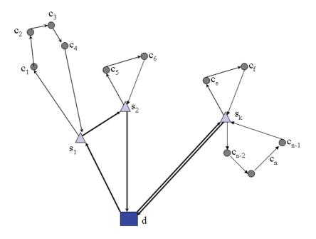
Figure 1: Example of 2E-CVRP transportation network
