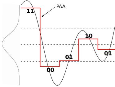
Fig. 1: Example of the SAX representation of a time series with  $N = 4$ . The dotted lines on the figure represent the three breakpoints of the Gaussian distribution  $\mathcal{N}(0, 1)$ . SAX symbols are represented by their binary values.
