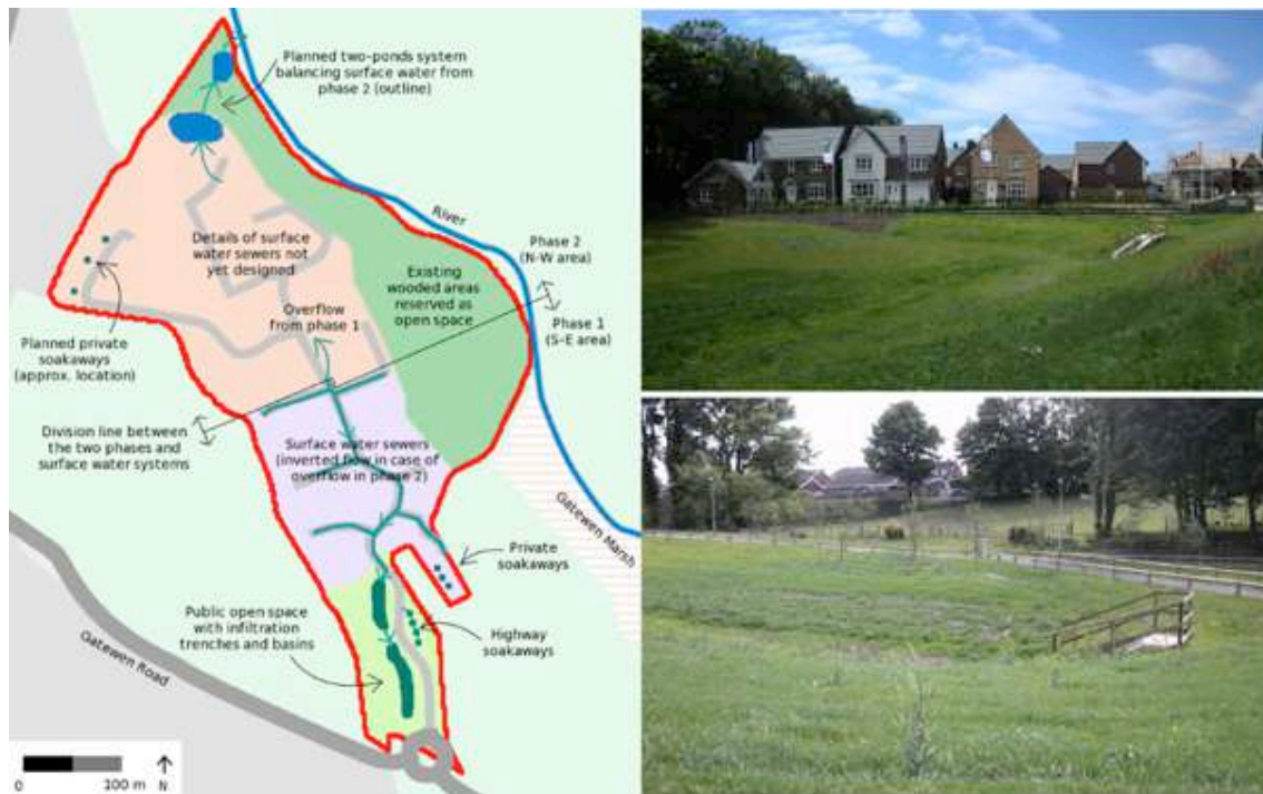
Figure 21. Stormwater management systems for Gatewen Village and photos of the basins and detention and infiltration trenches in the southwest zone (above: upper section; below: lower section).
