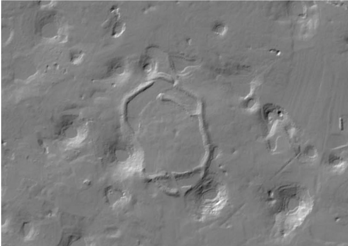
fig. 2. Feature detection using LIDAR under forest canopy : DTM showing dolines and fortification footprints in KRAS area, Wertern SLOVENIA. Source K. OSTIR.
