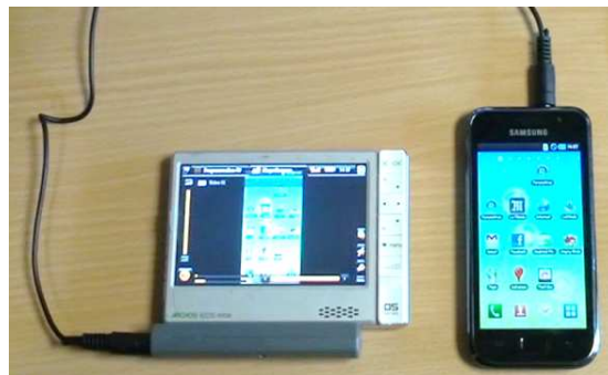
Figure 1. A simple portable set-up to record the audio-video flux on Android-based smartphones
