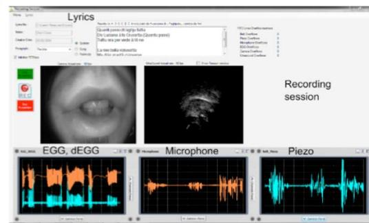
**Fig. 2:** Screen snapshot of the recording session software [10]. *Top:* display of Cantu in Paghjella lyrics. *Below:* 5 streams of the corresponding sensors, from left to right and top to bottom: lips from the camera, tongue contour from the US, time signals from EGG, microphone and piezoelectric sensor.
