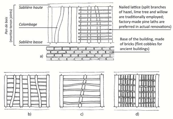
**Fig. 22.1** Examples of variability in timber frameworks from Northern France: (**a**) few spaced to moderately spaced laths, recorded in the Departments of Somme, Oise, and Pas-de-Calais; (**b**) *barreaudage* (horizontal bars) fi xed by notches on the timber framework, recorded in Haute Normandie and in western Oise; (**c**) *gaulettes* (thick and spaced bars), recorded in Normandie (Marais Vernier); (**d**) Flemish vertical wattle, that can be horizontal in some areas of Pas-de-Calais.
