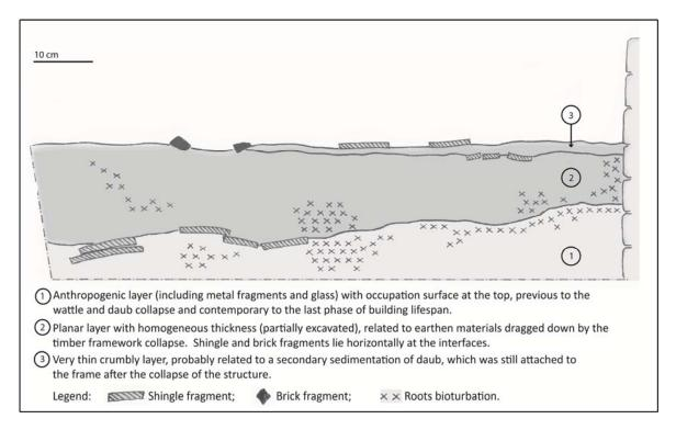
**Fig. 22.3** Partial cross section of a planar layer resulting from the collapse of a wattle and daub barn (Cf. Fig. 22.5a ) in Bainast-Les Alleux (Somme).
