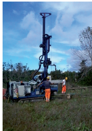
Fig. 4 : Mechanical corer (Core CPO-3) in the field on the Isola Sacra (F. Salomon).
