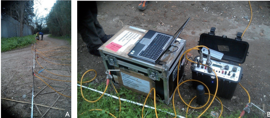
Fig. 3 : (A) Setting out of the ERT probes and checking on the Tigre ; (B) The Allied Associates Tigre Resistivity meter during the ERT survey (K. Strutt).
