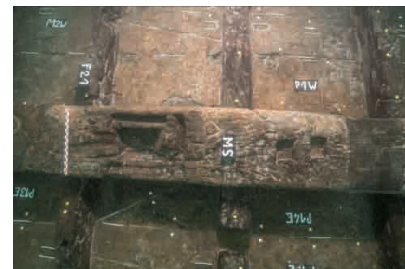
Fig. 10: The mast-step and the square stanchion recesses on the keelson (photo: T. Seguin)
