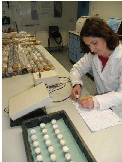
Figure 3. Using a Bartington MS2 magnetic susceptibility meter and MS2C dual frequency sensor.
