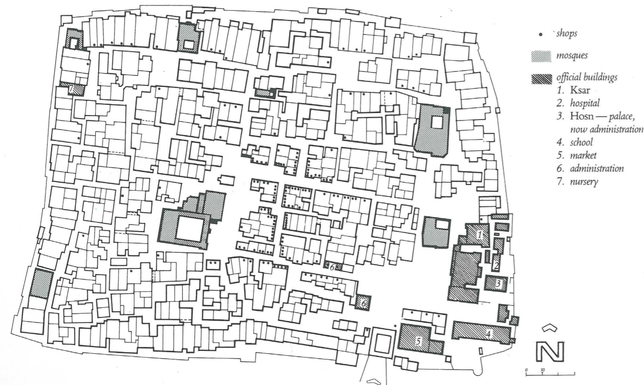
Site plan of the city of Shibam, South Yemen. Indicated on the plan are institutional buildings, commerce, mosques and residences.
