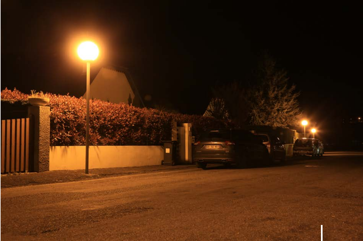
Full cut off lights; high pressure sodium lamps; 2200 °K; 6 lux.
