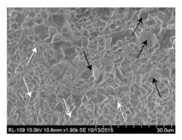
**SOM Figure S3.** Back-scattered electron image of the sample. Observations show that the carbon is mostly in the form of tiny balls, about 2  $\mu$ m in diameter, which is a common form for soot (Tomasini et al., 2012). White arrows = some representative tiny balls of soot, black arrows = some representative calcite crystals. The upper and lower parts of the image show more soot than the central part, where carbonate crystals are best seen.
