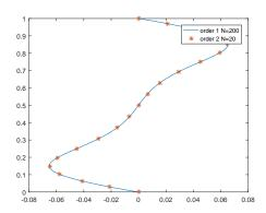
FIGURE 10. Comparison of the horizontal velocity profile u(y) at mid-domain x = 0.5 between the scheme (5.8) and [11].
