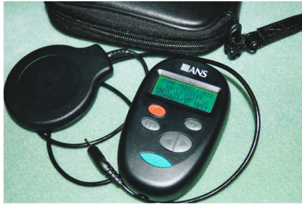
Figure 2: the remote control together with the coil and the leather case
